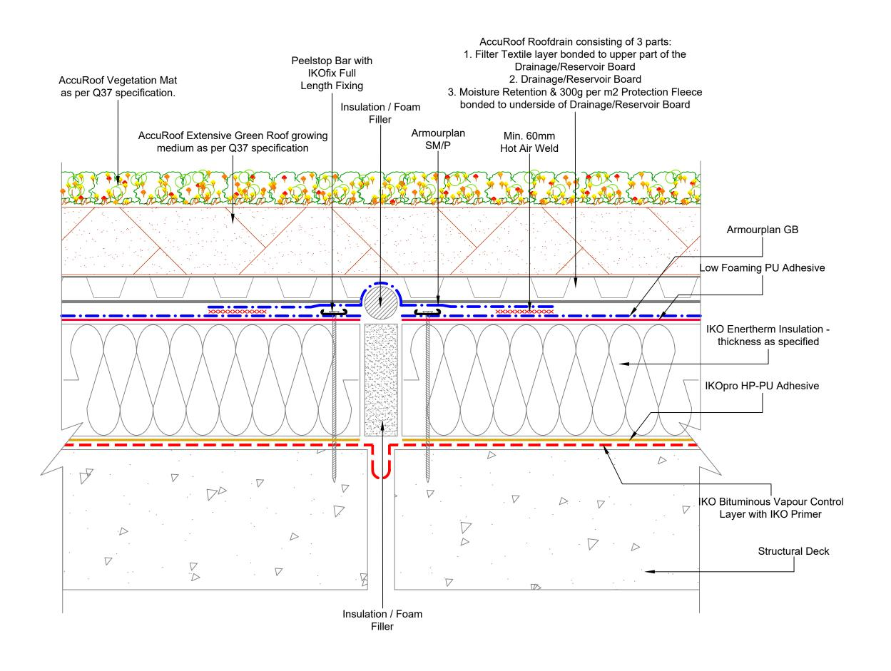
The Waterproofing System should be installed in accordance with BS6229:2018 and AccuRoof project Specification.
