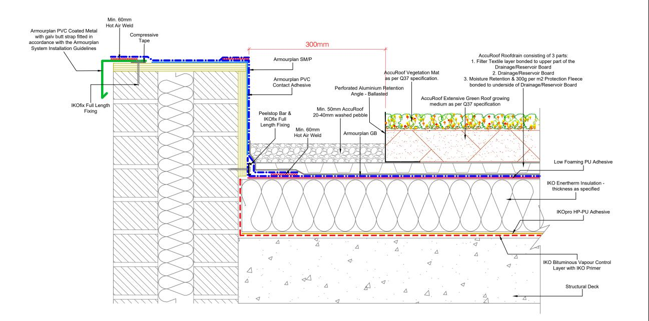
The Waterproofing System should be installed in accordance with BS6229:2018 and AccuRoof project Specification.
