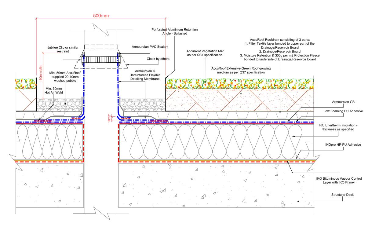
The Waterproofing System should be installed in accordance with BS6229:2018 and AccuRoof project Specification.
